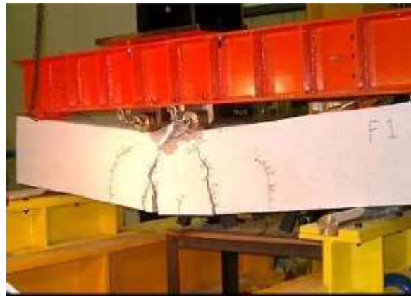
Flexural Cracks in Beam
