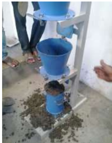
Compaction Factor Test
